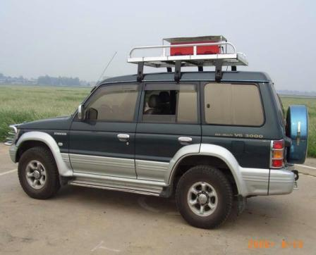
The CGS system was installed in jeep, with large volume(4L) , GR460 , Nal(TI) detector.
